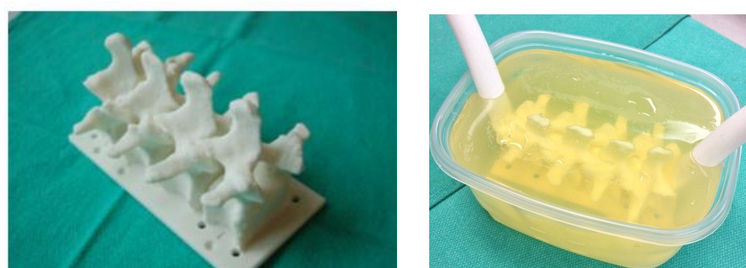
Figure 2. Spinal phantom. Four tissue types were simulated: spinal chord, ligamentum flavum, fat and skin.
